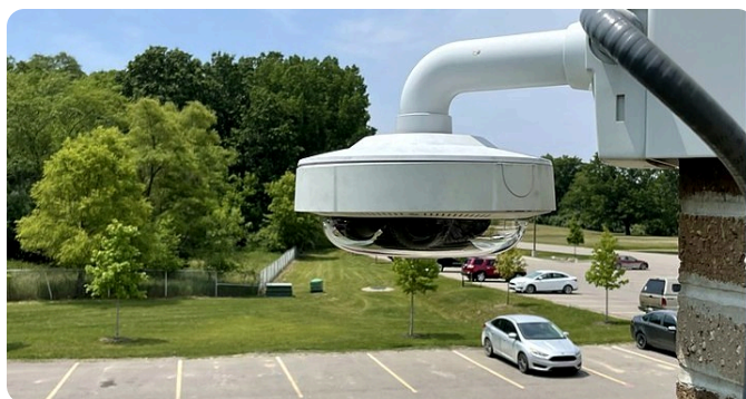
A multi-sensor camera covering an entire parking lot from one mount.
